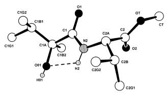
**Fig. 5** X-Ray diffraction structure of H-L- $(\alpha Me)$ Hyv-L-Val-OMe with numbering of the atoms. The intramolecular H-bond is indicated by a dashed line.
