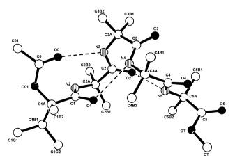
**Fig. 7** X-Ray diffraction structure of Ac-L-(αMe)Hyv-(Aib)<sub>4</sub>-OMe with numbering of the atoms. The three intramolecular H-bonds are indicated by dashed lines.
